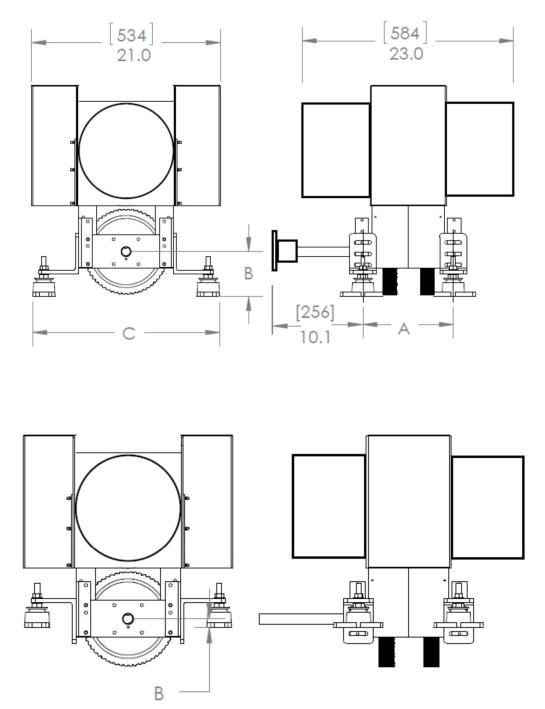
A) Center Line of Foot to Center Line of Foot 8"(203) Min 11"(279) Max B) Center of Shaft to Above shaft 1.65"(42) to 6.2"(157) Below Shaft C) Outside to Outside of Foot Min 16.4"(416) Max 20.8"(528)
